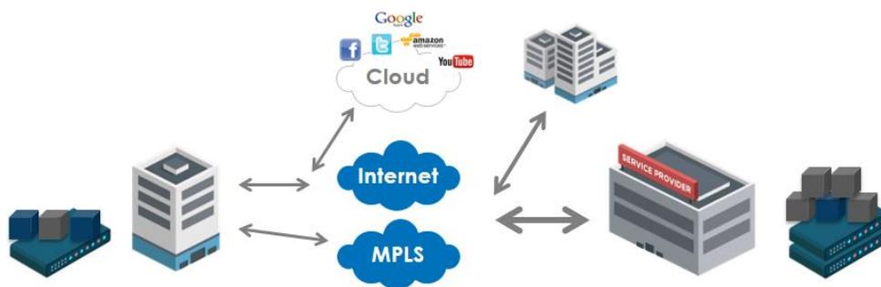
Taking an example of SD-WAN, imagine an enterprise with 400 branch offices that wants to utilize inexpensive, high throughput broadband connections as an element of its overall WAN architecture. Instead of purchasing legacy routers and firewall appliances and shipping them to branch sites, the
